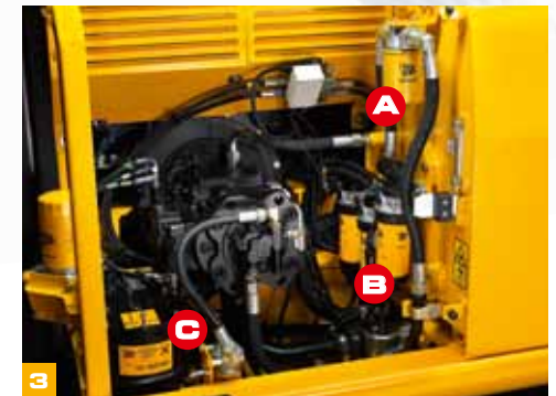
(A) Hydraulics oil filters (B) Fuel filters (C) JCB Plexus Oil Filter System
