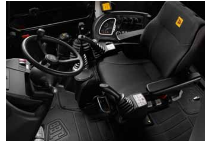
Precision Control system with integrated, seat-mounted controls
